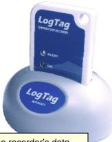
Read & save the recorder's data by simply placing it into the reader. Available in USB or Serial Version.
